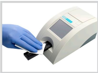
Figure 8: Cleaning the REF pad on the strip holder tray
