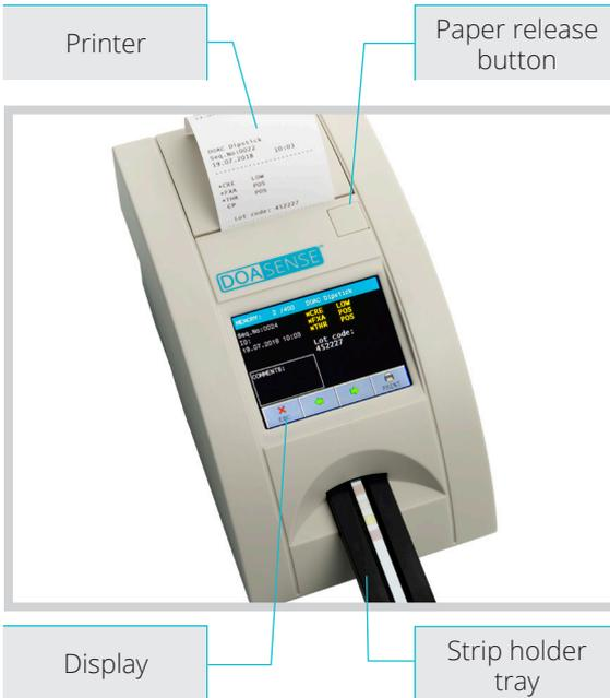
Figure 2: Description of the front part of the instrument
