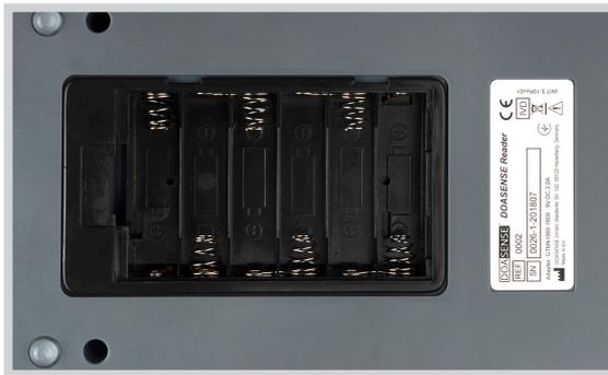
When batteries (type LR6) are used, 200 measurements with printing or 240 measurements without printing can be made with one set of batteries. The instrument displays a BAT icon on the LCD that gives information about the battery status.
